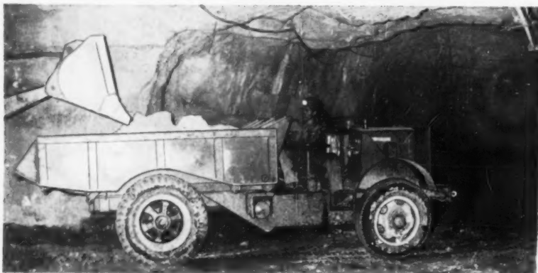
SCOOT-CRETE CD-4, shown being loaded in mine, will carry up to 15 tons payload. Model CD-3N has 5-ton payload. Note driver's side-mounted position for maximum vision and efficiency, forward and rear.
